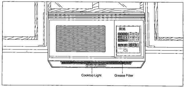
The exhaust hood feature on your Panasonic microwave oven is equipped with a metal filter which collects grease as air is drawn up through the filter.
