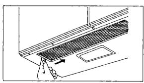
To remove grease filter, grasp the "knob" on the filter and slide filter to the right. The filter will drop out.
