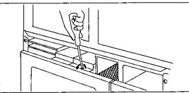
Step 4. Unscrew bulb and replace only with 115-125 V, 20 W bulb. Do not use more than 20 W bulb. If this bulb is not available locally, contact the nearest authorized Parts Distributor.
